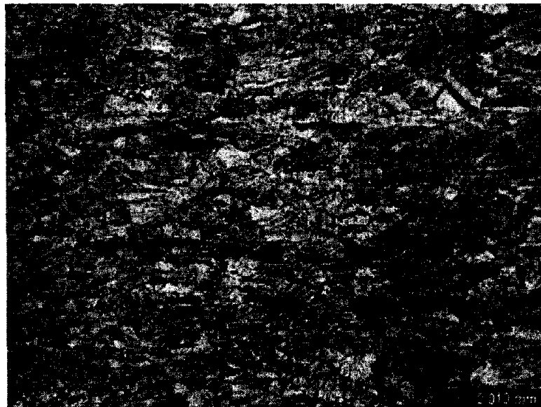
Figure 2. Optical micrograph of Cu-Be alloy heated at 410° C with a belt speed of 11.25 in/min at Agilent Technologies, with some polarized light and color enhancement.
