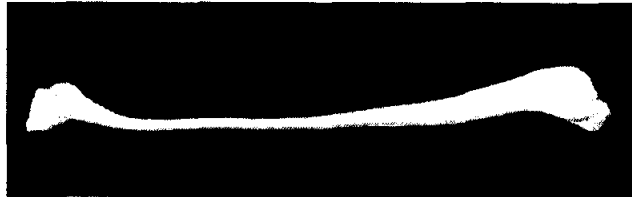
Figure 12: Stretched out Silly Putty, greatly deformed at a low rate, without breaking.
