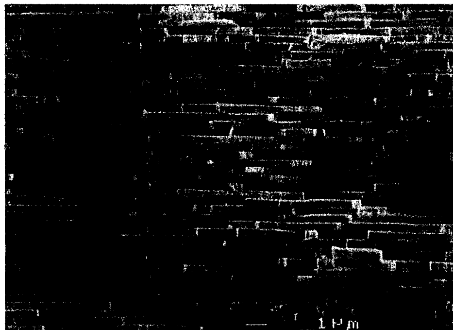
SEM image of a cross section of native gastropod (red abalone) nacre
