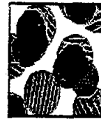
Figure 5. Solidification of a 10% B alloy. Proeutectic B is growing and the eutectic (A + B) is beginning to form.
