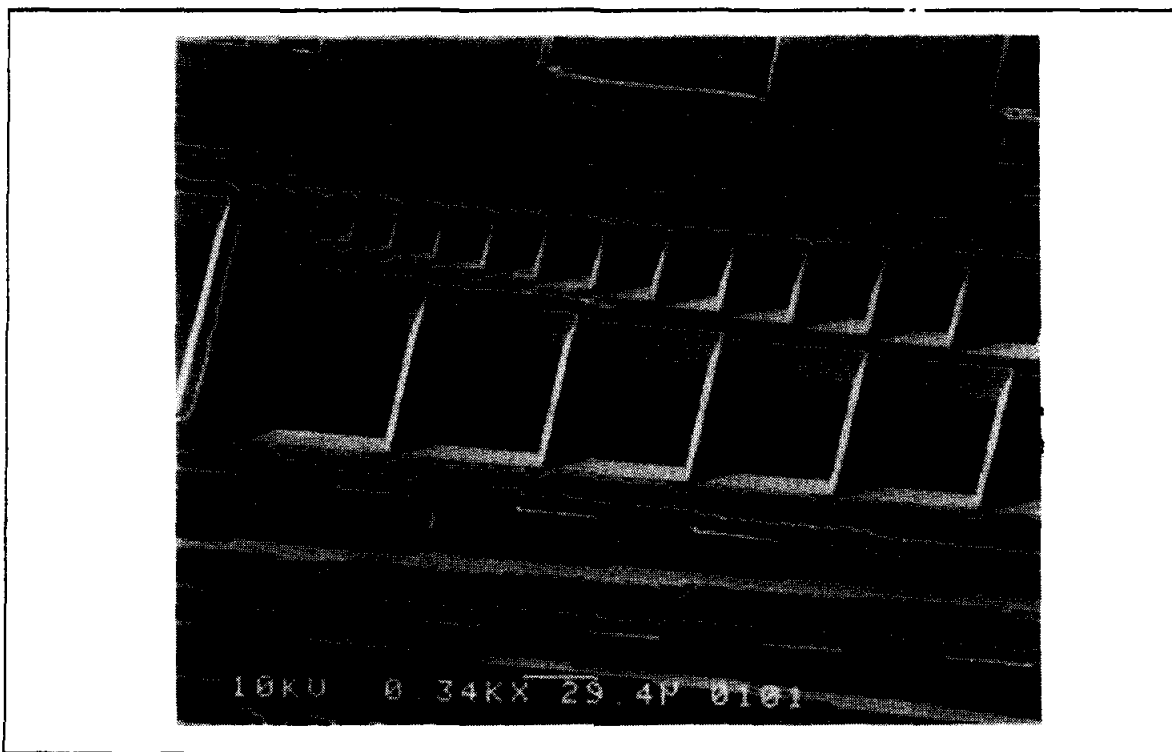
Figure 9. An example of etch results using KOH for 2.5 minutes. The largest completely etched pit is 19x19 \mu\text{m} .
