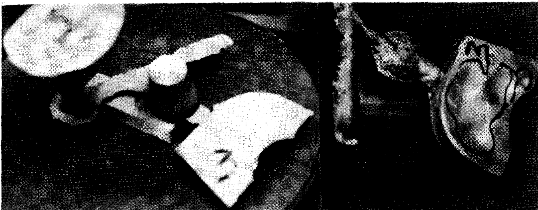
Figure 8. An unsuccessful casting using a medium riser and containing bottom shrinkage. The riser connection was not completely open and froze prematurely.
